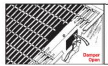
Setting No. 1 - In mild weather, operate furnace with damper open. Furnace will cycle on and off maintaining a moderate grill temperature and an even room temperature.
