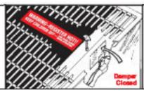
Setting No. 2 - In extremely cold weather, close damnper (which exposes hot register warming plate). Furnace will then put out maximum amount of heat until room temperature reaches setting on wall thermostat.
